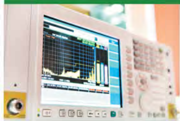
Receiver for measuring electromagnetic field
