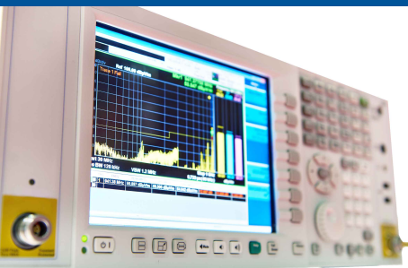
Receiver for measuring electromagnetic field
